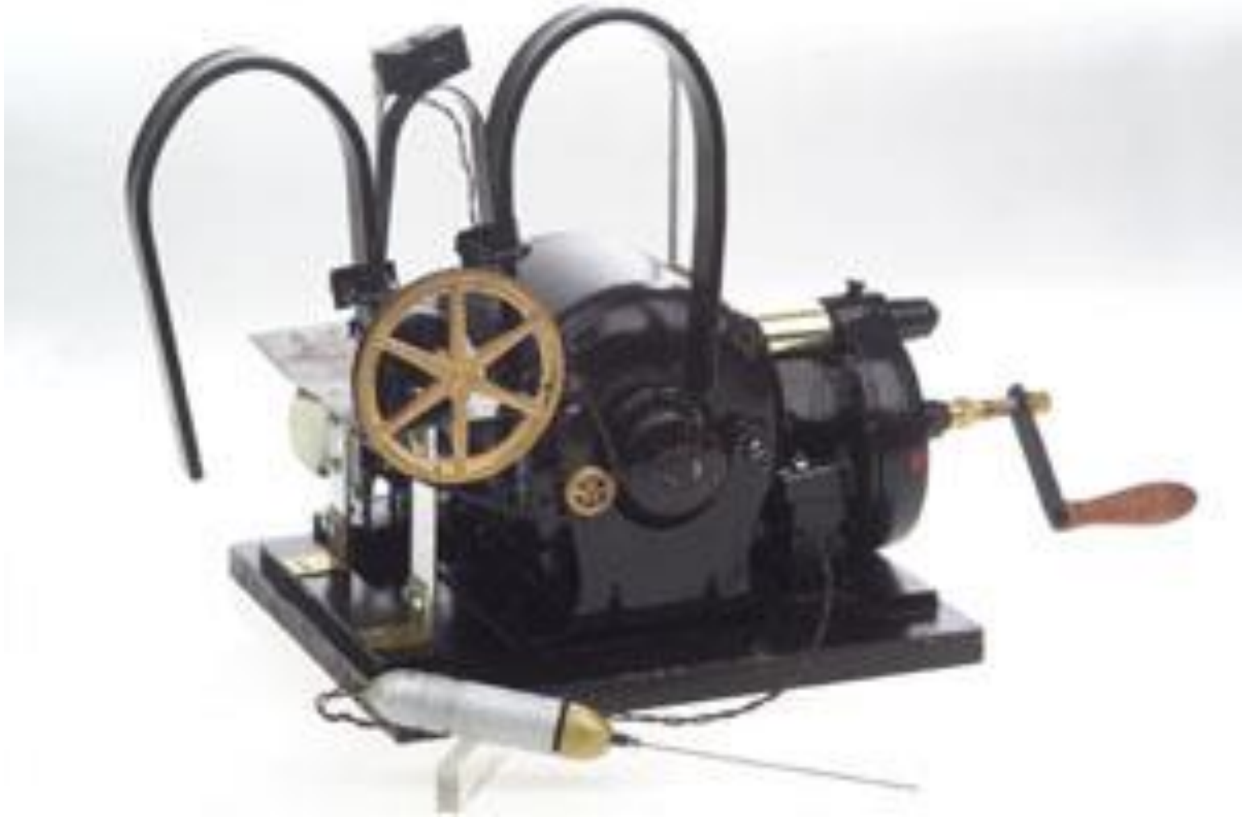
Reconstruction of the first „artificial“ pacemaker with crank and spring-driven pulse generation (A.S. Hyman, 1932)
