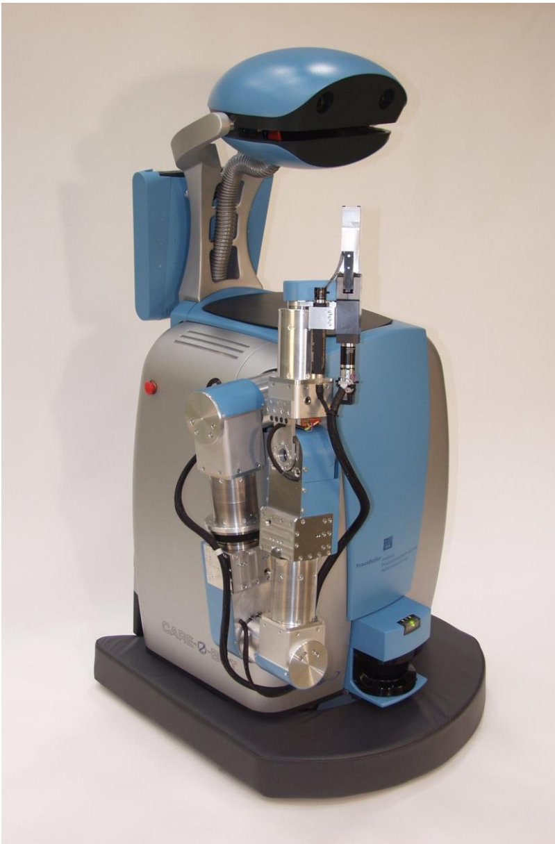
Two Care-O-bot robots for home-nursing (Fraunhofer Institute IPA), remote control (key board, voice), autonomous intelligence, sensors (orientation, movement)
