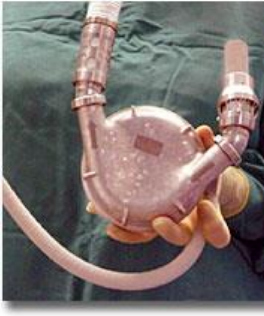
Left ventricular assist device LVAD with hydraulic pumping
