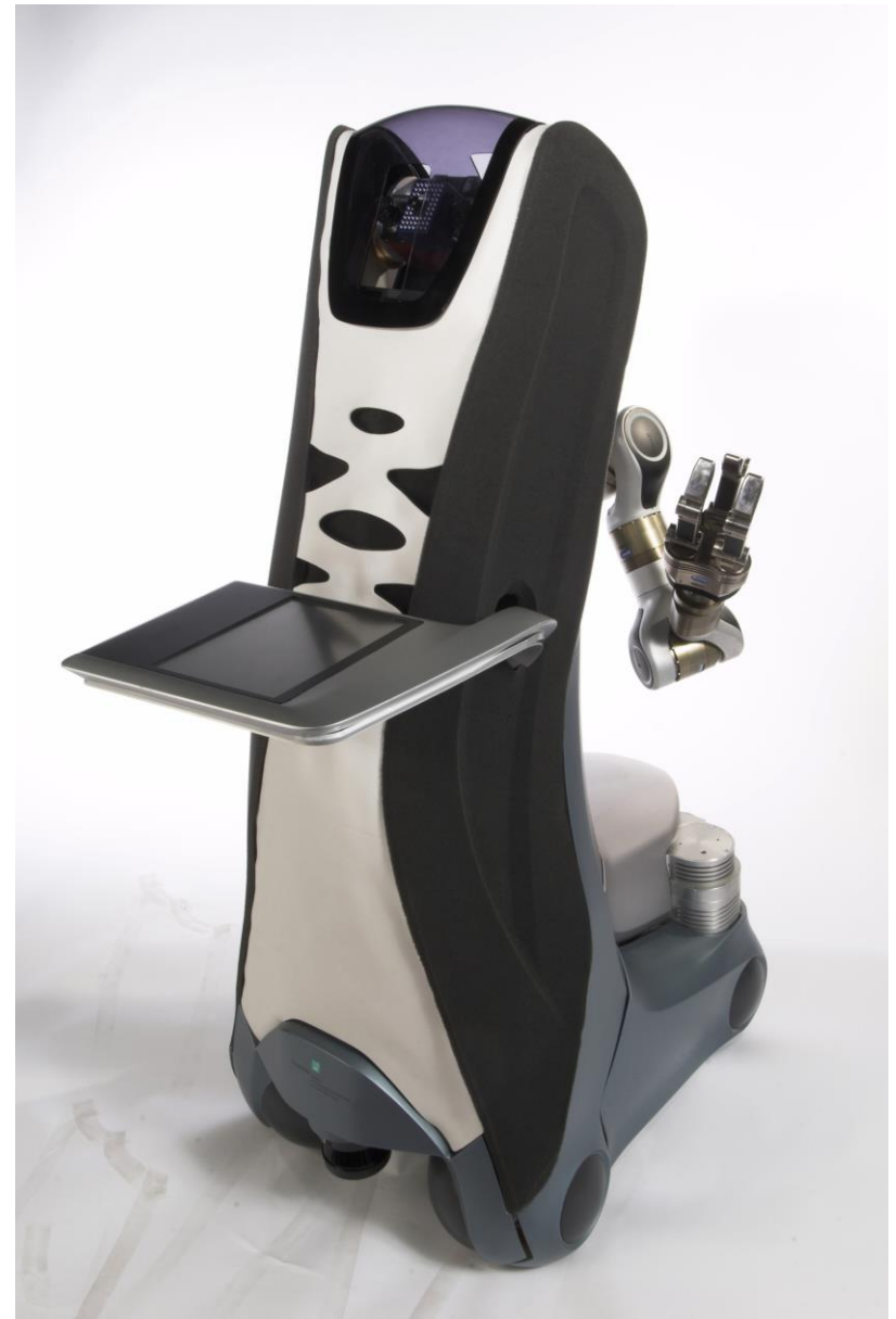
Two Care-O-bot robots for home-nursing (Fraunhofer Institute IPA), remote control (key board, voice), autonomous intelligence, sensors (orientation, movement)
