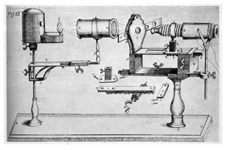
Microsope with horizontal beam path and burning candle as "light source" (1691)
