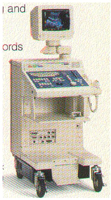
Multipurpose ultrasonic imaging apparatus for colour flow mapping (Aloka 1990)
