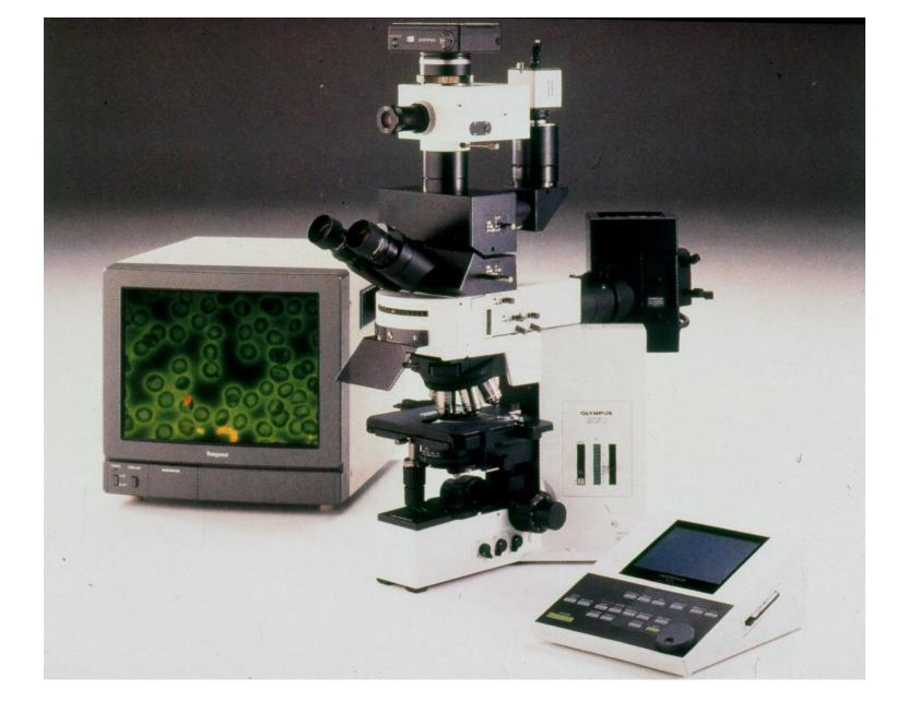
Microscope with computer-assisted image processing and presentation
