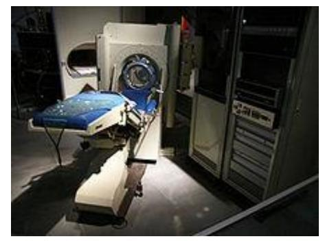
*Upper left*: Reconstructed laboratory equipment of the EMI-Hounsfield-CT-Scanner with an isotope source, sampling time 9 days
