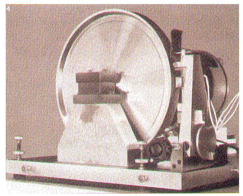
Memory wheel (diameter 40 cm, 50 revolutions per second) for video recording, Philips (1957)
