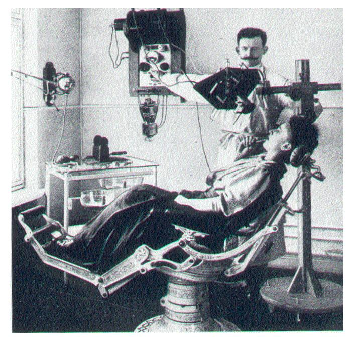
X-ray testing of jaw and teeth with free running cables (Siemens 1911)
