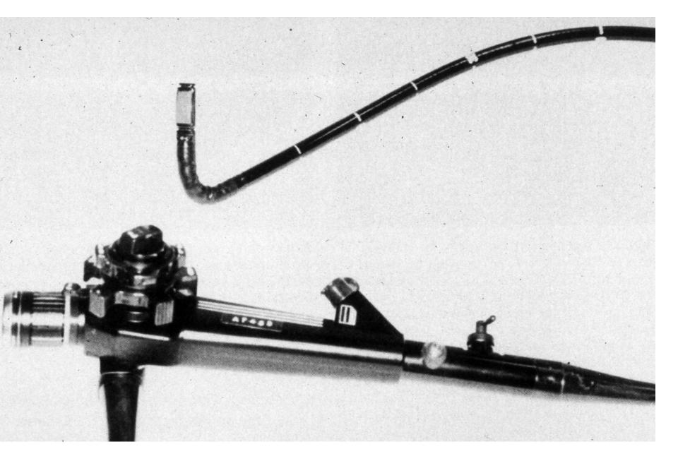
Actively bendable (flexible) endoscope with imaging and working channel (1980)
