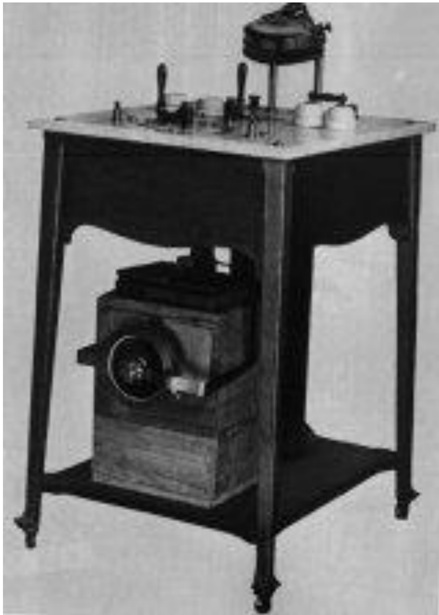
Apparatus for electrotherapy (d'Arsonvalisation, diathermy)
