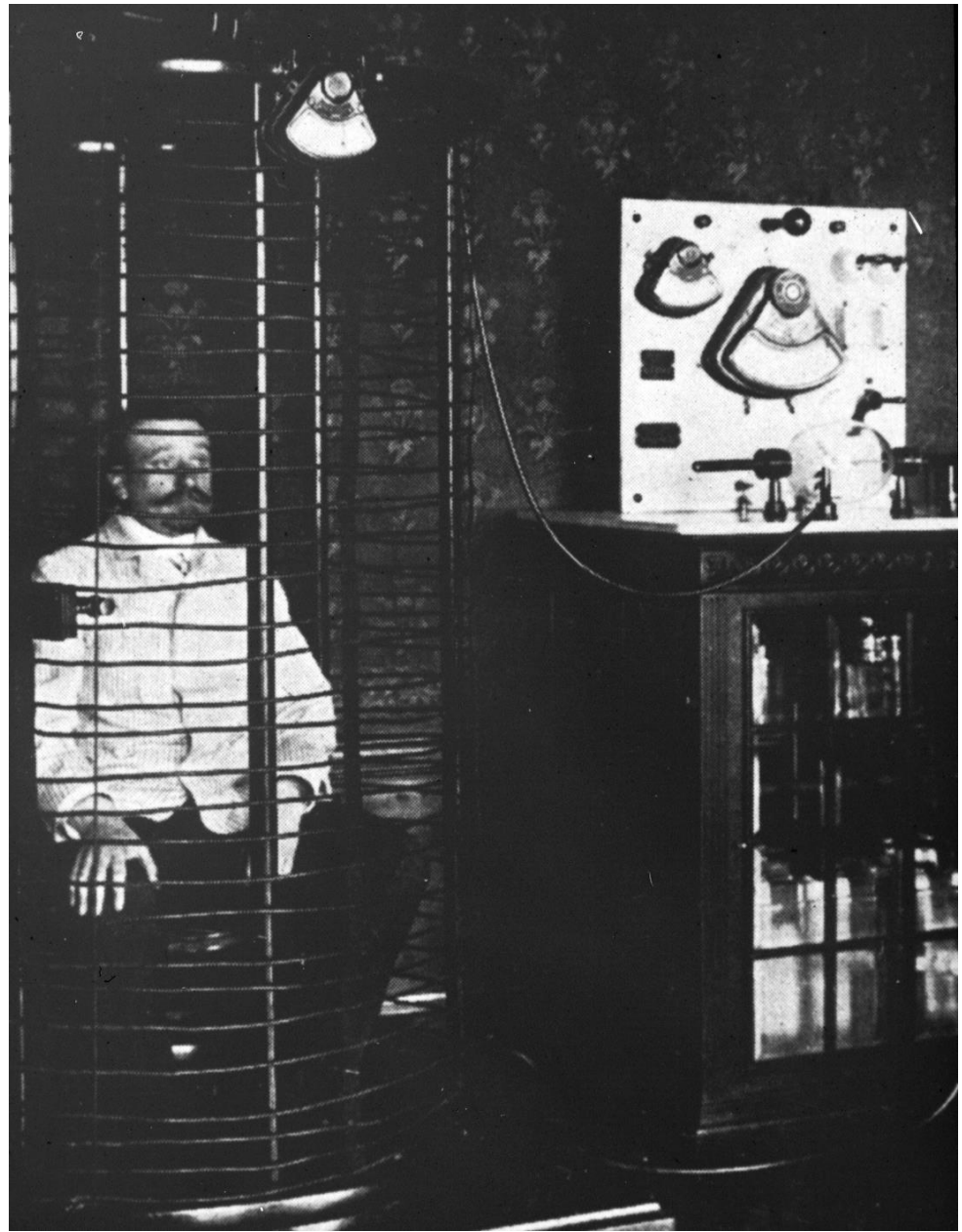
Solenoid for magnetic stimulation: Schematic and experimental arrangement (J-A. D'Arsonval himself?, 1893, based on research work by N. Tesla)
