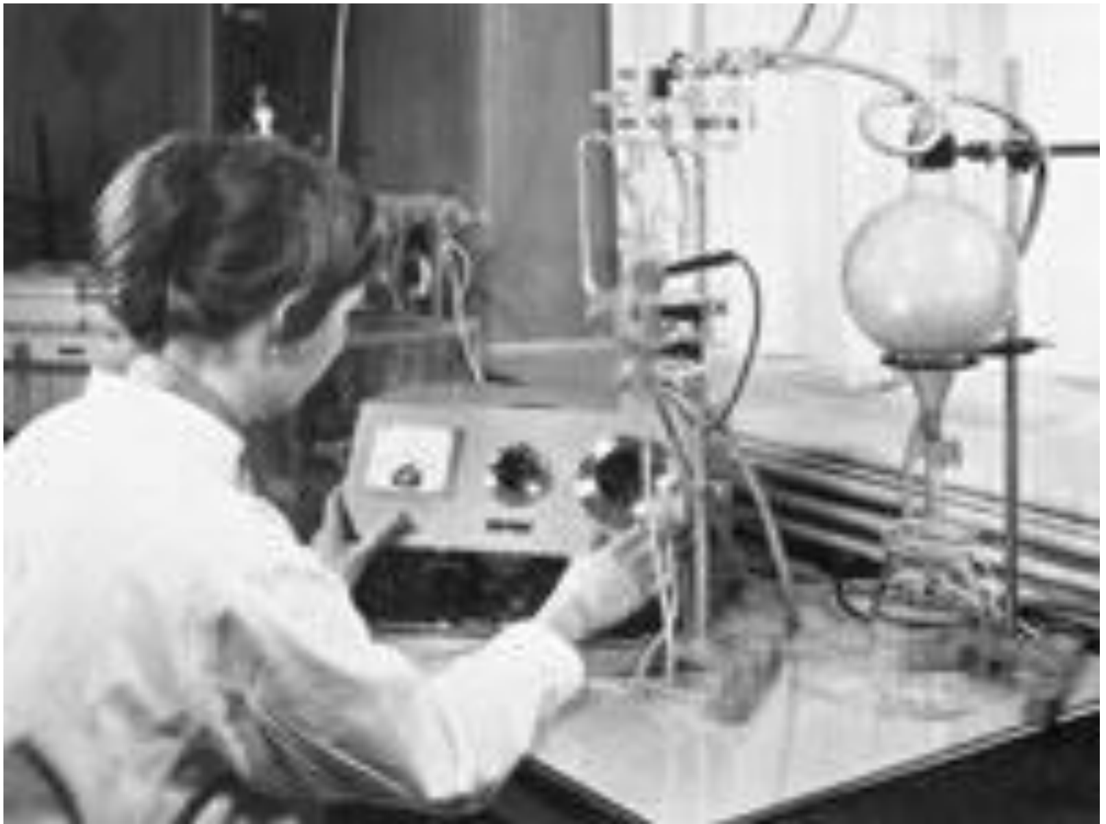
The first appliance for the measurement of the pH-value in blood (Radiometer, 1952)
