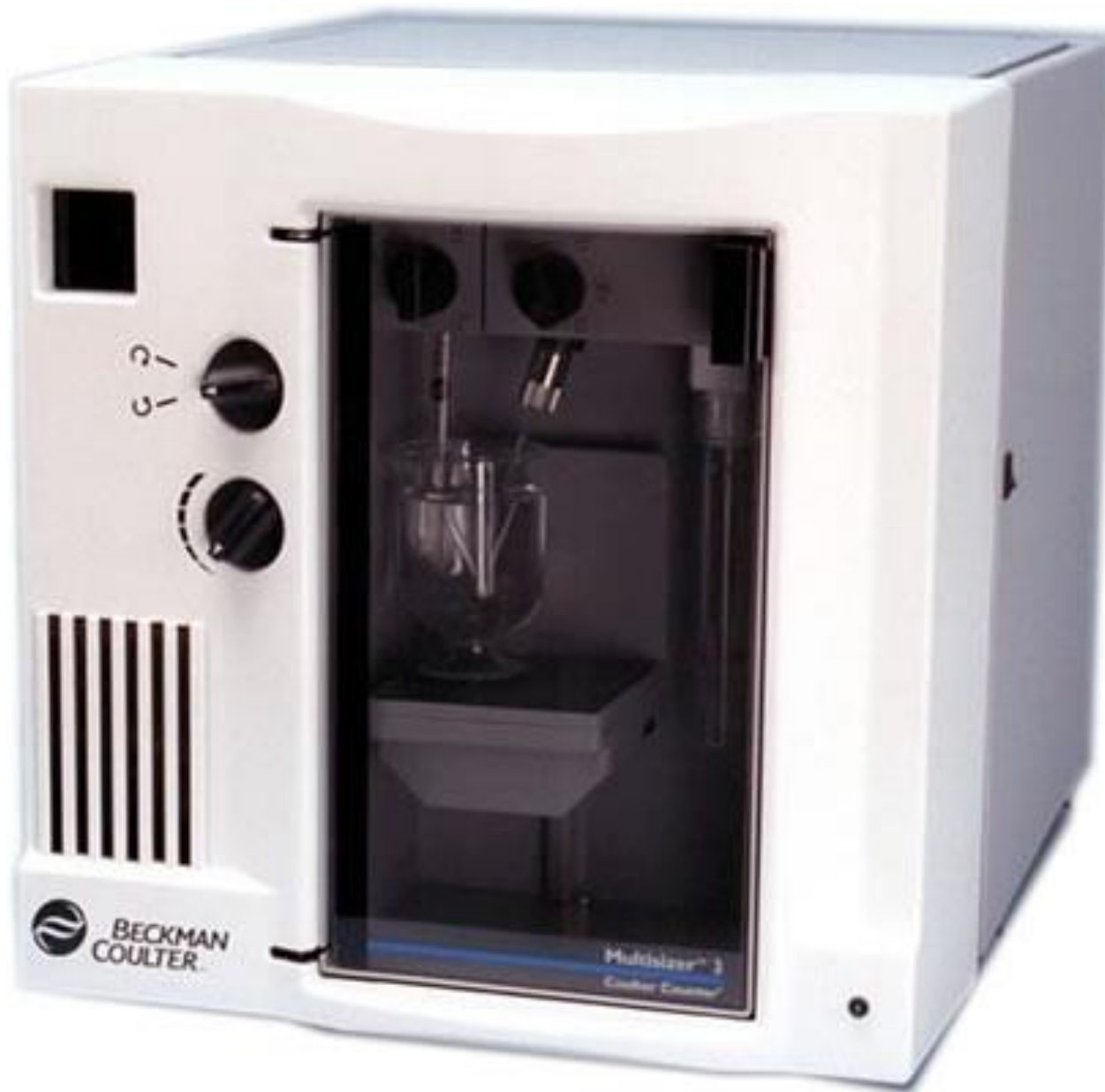
Automated blood cell counter ( W.H. Coulter , 1947), based on impedance measurement
